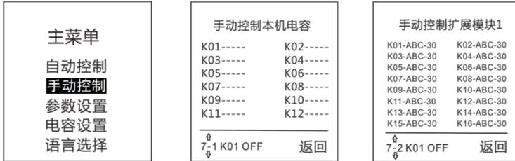
On the Main Menu screen, press + and - to select the manual control menu item, and press M to enter the Manual Control screen. Press +, -, ←, and → To move the cursor, you can select and switch capacitors on the local device or expansion module. Move the cursor to the right and press M to return to the main menu.
