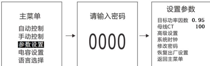
1, the target power factor: the user wants the system to reach the normal power factor value. The default value is 0.95.
