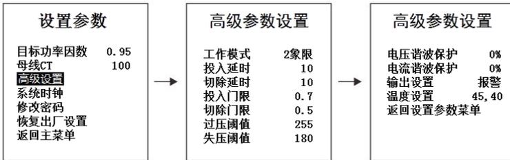
1. Working mode: working quadrant setting. Power generation system compensation option 4, other compensation option 2. The default value is 2.
